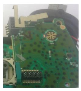
Make sure that the connections on the Arbiter 4 chip are solid and not dry joints. It is easy to make dry joints that appear good but break very easy. If you get dry joins the chip will not work.
