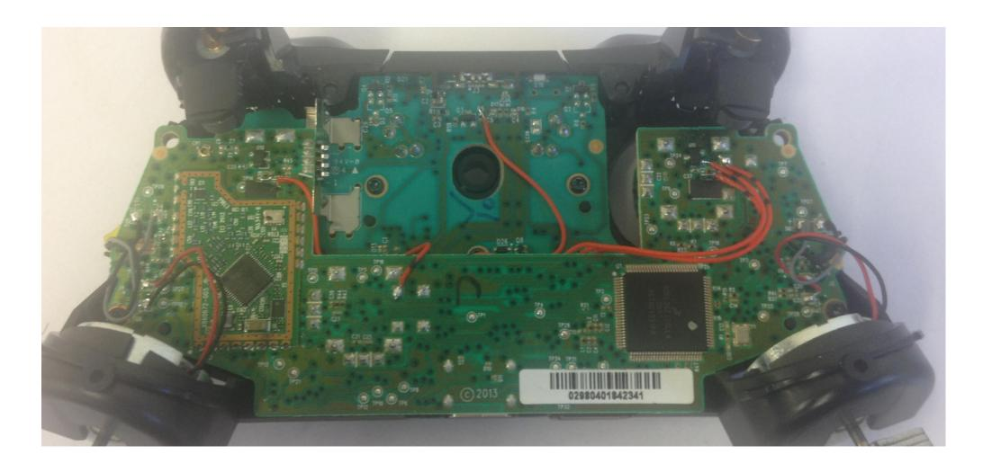
Note that for the RT and LT connections, the bottom pin of the resistor (left) and capacitor (right) are joined, so you are ok to connect the wire going over both pins like we do.
